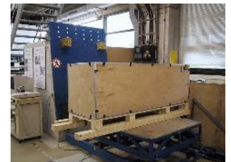
Horizontal shock resistance test
